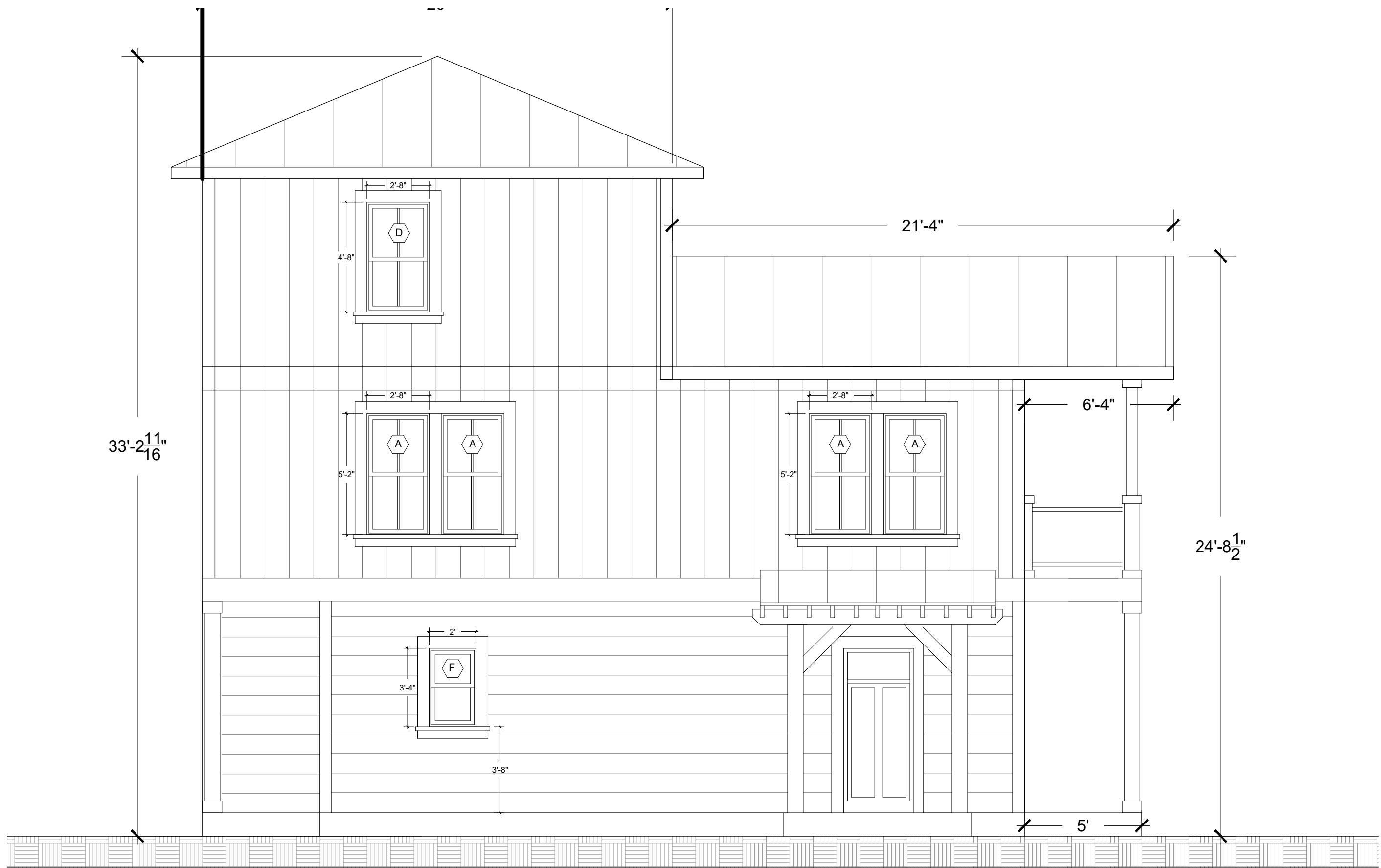
4 UNIT-2 SIDE ELEVATION- NORTH SCALE: 1/4" = 1'-0"
