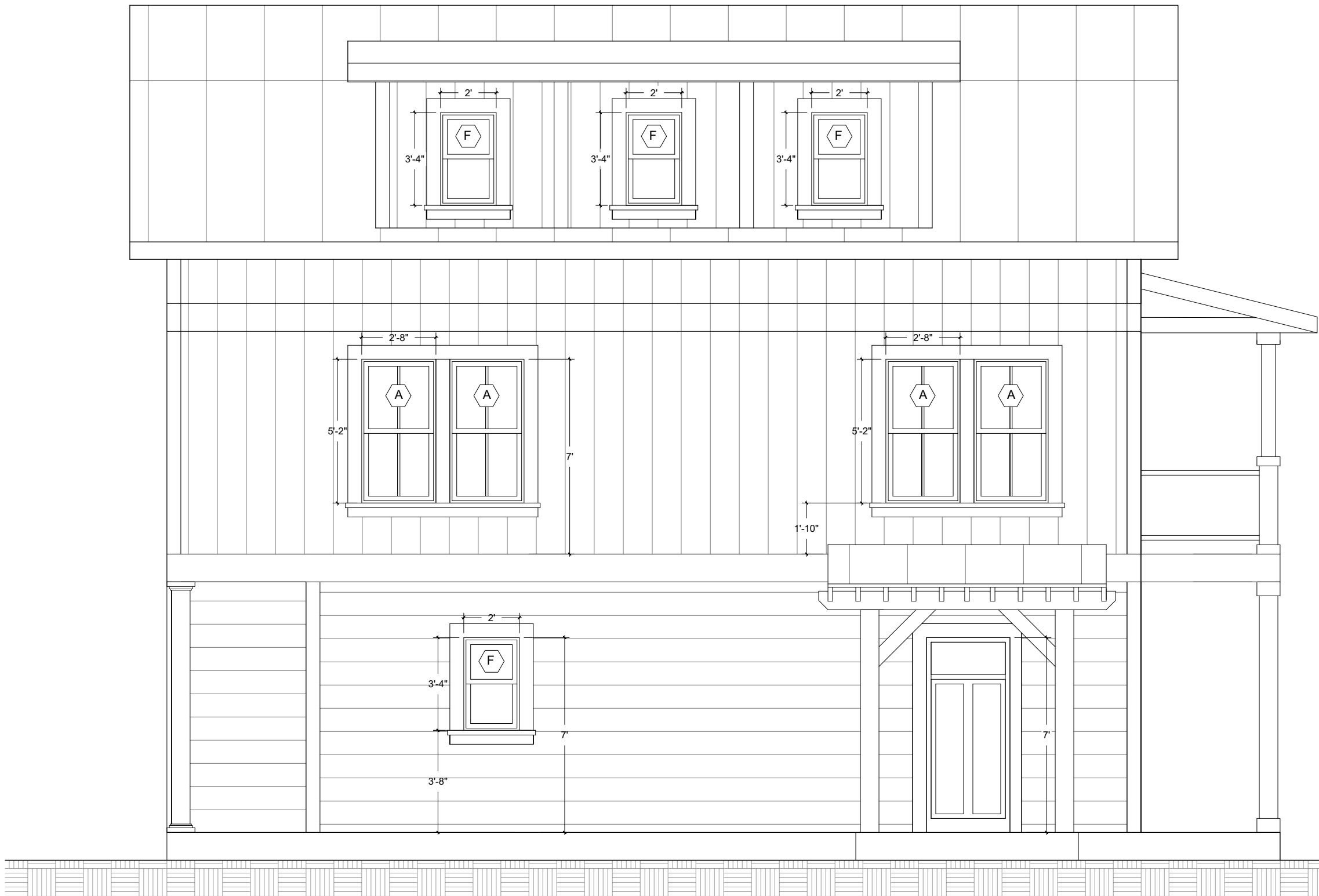
4 UNIT-3 SIDE ELEVATION- NORTH SCALE: 1/4" = 1'-0"
