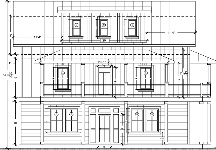
1 UNIT-1 FRONT ELEVATION- NORTH SCALE: 1/4" = 1'-0"
