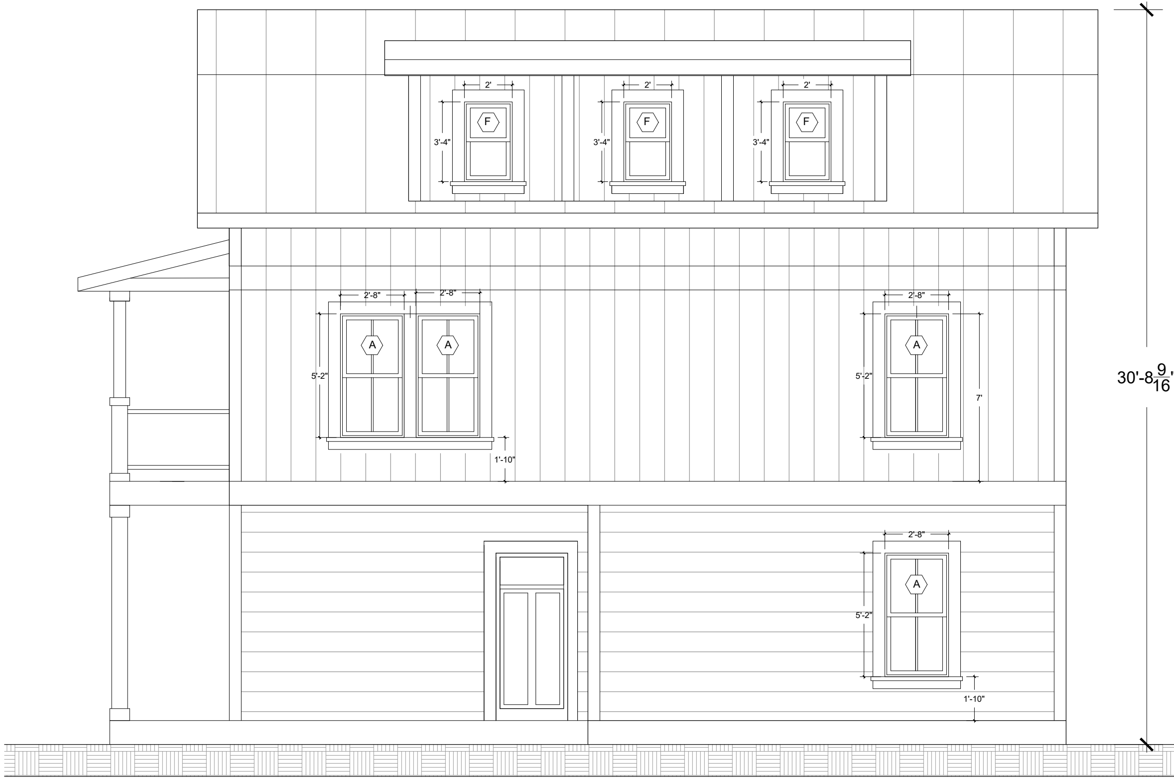
2 UNIT-3 SIDE ELEVATION- SOUTH SCALE: 1/4" = 1'-0"
